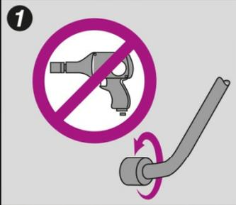
1 Do not use an air impact gun for installation!
