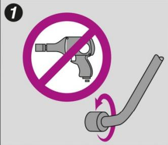
Do not use an air impact gun for installation!
